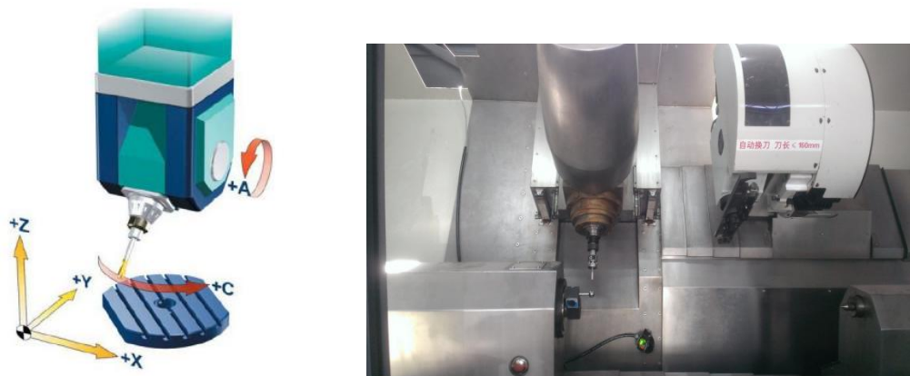
Figure 2-3 Mixed structure machine tool
