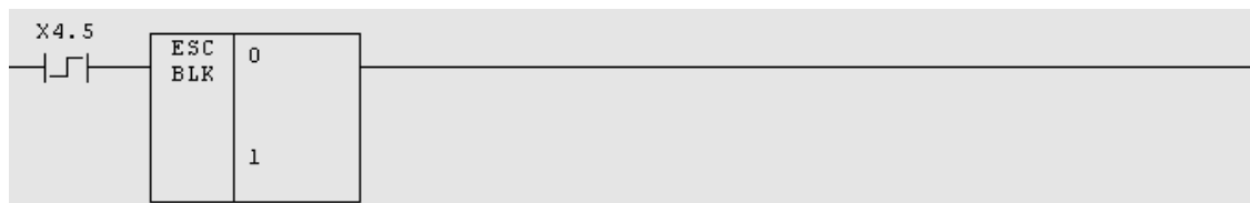
Figure 2 Activation of G31 block skip command
