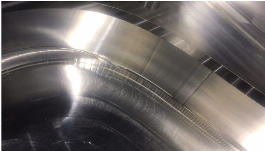
Figure 3-11 S-shaped piece with machining defects
