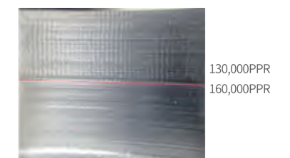
Quality difference of machined surface
