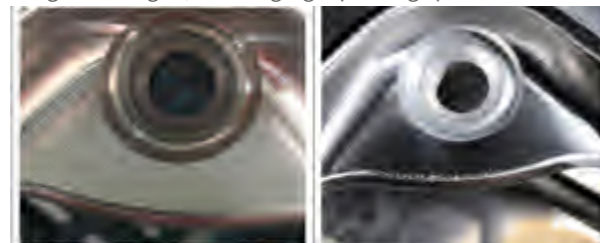
Overcut and chatter marks at corner
